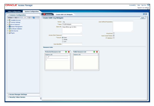
Specify a name for Webgate and the Base URL (the host and port of the computer on which the Web server for the Webgate is installed). Click 'Apply' button.
